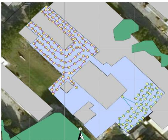
When this option is activated, a line is drawn between the measurement points in their order of acquisition. The objective is to **make it easier the detection of possible GPS jumps and to better interpret the measured values when the trajectories intersect**. A different color is assigned to each campaign.
