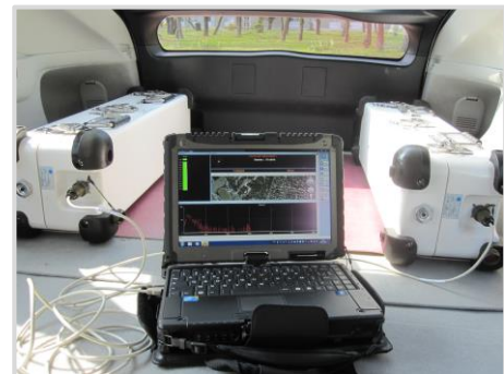
Embedded in a vehicle, IRSN Ulysse gamma spectrometry system maps radionuclides over large areas
