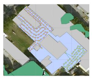
When this option is activated, a line is drawn between the measurement points in their order of acquisition. The objective is to make it easier the detection of possible GPS jumps and to better interpret the measured values when the trajectories intersect. A different color is assigned to each campaign.
