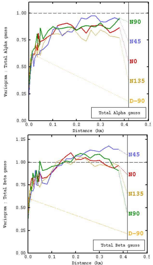
Fig. 5 Experimental variograms for Gross Alpha and Gross Beta, computed for the vertical direction (D-90) and four horizontal directions (N0 to N135).
