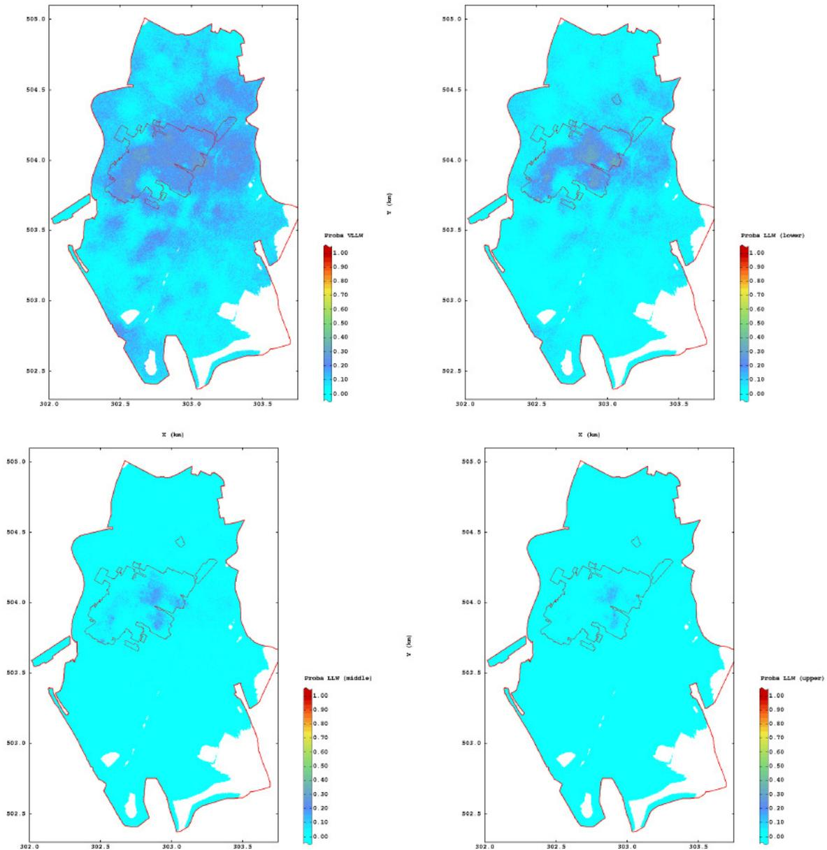
Fig. 8. Plan section of the area within the Sellafield site boundary for the first layer of grid cells below ground elevation. The probabilities of cells in this layer belonging to particular soil classes are shown: 'VLLW' (top left), 'LLW lower' (top right), 'LLW middle' (bottom left) and 'LLW upper' (bottom right). White areas are not interpolated due to the neighbourhood
