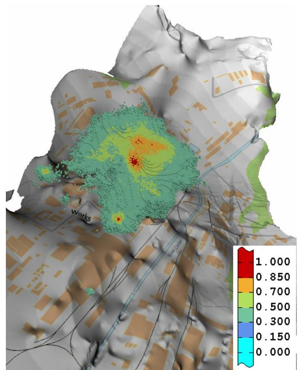
Fig. 10. Probability to exceed 18,000 Bq/m<sup>3</sup> in groundwater (only cells with probabilities greater than 30% are displayed). The 3D view shows an area within the Sellafield site boundary: compare with Fig. 3 to get the location
