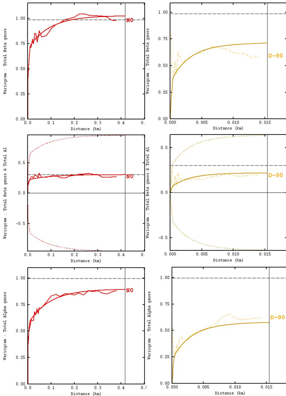
Fig. 6. Experimental variograms (left: horizontal, right: vertical) and corresponding model for Gross Alpha (bottom), Gross Beta (top) and the cross-variogram (middle).
