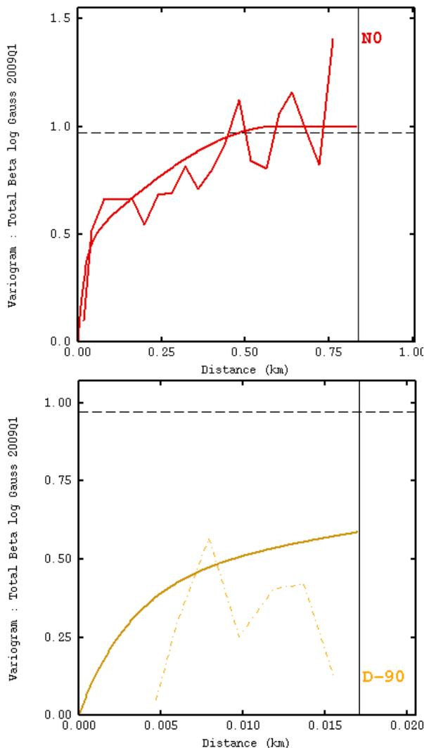
Fig. 9. Variographic analysis of the gaussian transform of log<sub>10</sub>(gross beta): Horizontal (top) and vertical (bottom) variogram.
