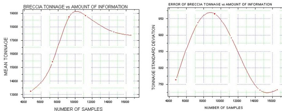
Figure 5. a) Average number of Simulated Breccia Blocks v/s Number of Drillhole Samples. b) standard deviation of the number of Simulated Blocks v/s Number of Drillhole
