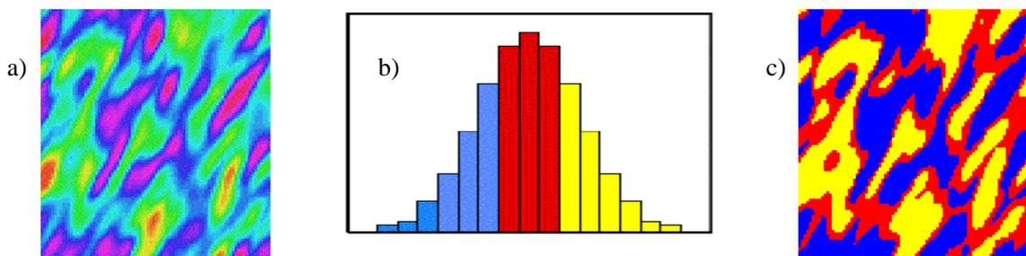
Figure 2. Principle of the Truncated Gaussian simulation method.
