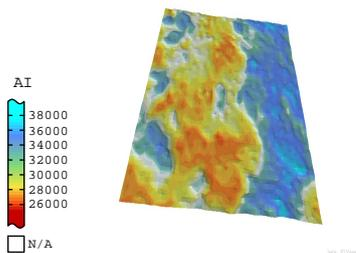
Figure 8: Map of the acoustic impedance after filtering.
