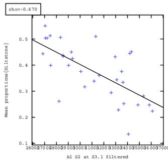
Figure 7: Scatter diagram between the average proportion of siltstone facies of the reservoir and the acoustic impedance filtered at the depth of a given intermediate horizon.
