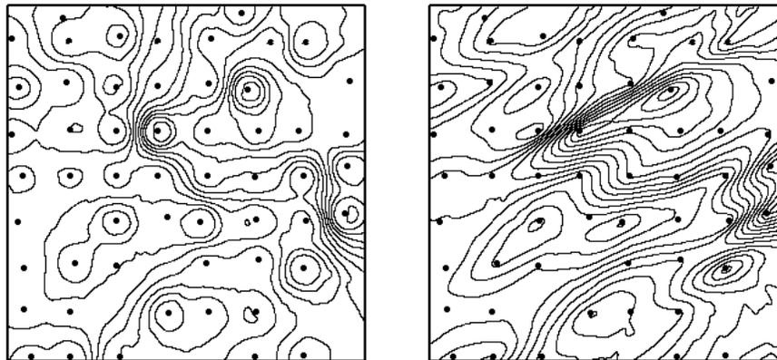
**Figure 4.** The difference between inverse weighted difference interpolation (left) and kriging (right) using a 3:1 anisotropic variogram model oriented N60E. The neighborhood search ellipse is identical for both.
