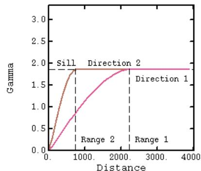
Figure 2. Anisotropic variogram showing a short-scale correlation range of 800 m and a long-scale range of 2200 m.
