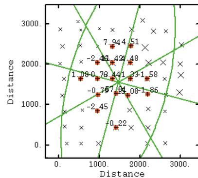
**Figure 3.** An anisotropic search ellipse with eight sectors and a maximum of two data points per sector. The minor axis has a length of 1000 m. The major axis (N15E) has a length of 4000 m. The center of the ellipse is the target grid node for estimation. There are 55 sample points (x) in the study area. Weights (in %) are shown for data control points used for estimation at the target point.
