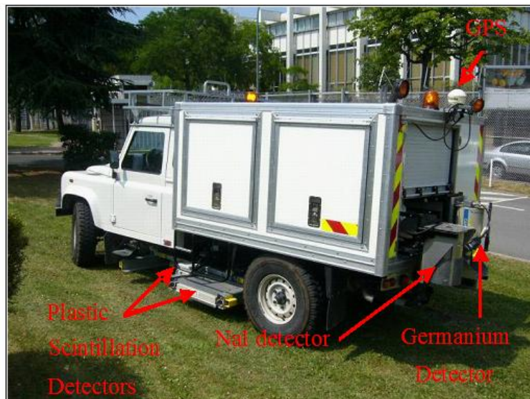
Figure 1: Real-time data acquisition on a CEA site with VEGAS expertise vehicle
