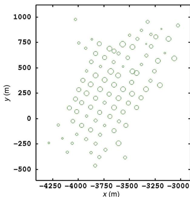
**Figure 1.** Distribution of exploratory boreholes in the study area. Boreholes are located in regular grids with an average spacing of 100 m.
