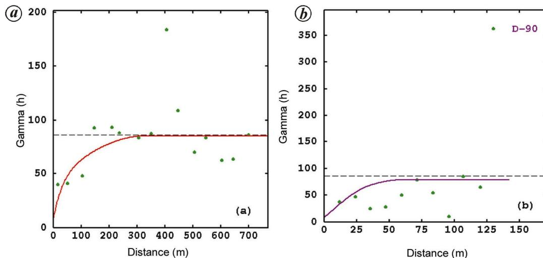
**Figure 7.** Omni-directional semi-variogram models of Fe% for domain B in horizontal direction (a) and vertical direction (b). Both the semi-variograms show reasonably good spatial structure with nested models.
