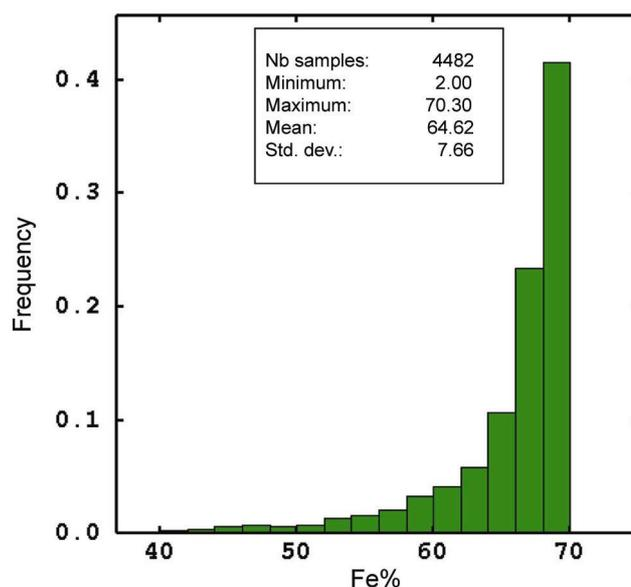
**Figure 2.** Histogram showing grade distribution of Fe% in the borehole samples. Majority (85%) of the samples exhibit Fe grade >60%; 9% of samples exhibit 50–60%, and the remaining samples exhibit <50% Fe grade.
