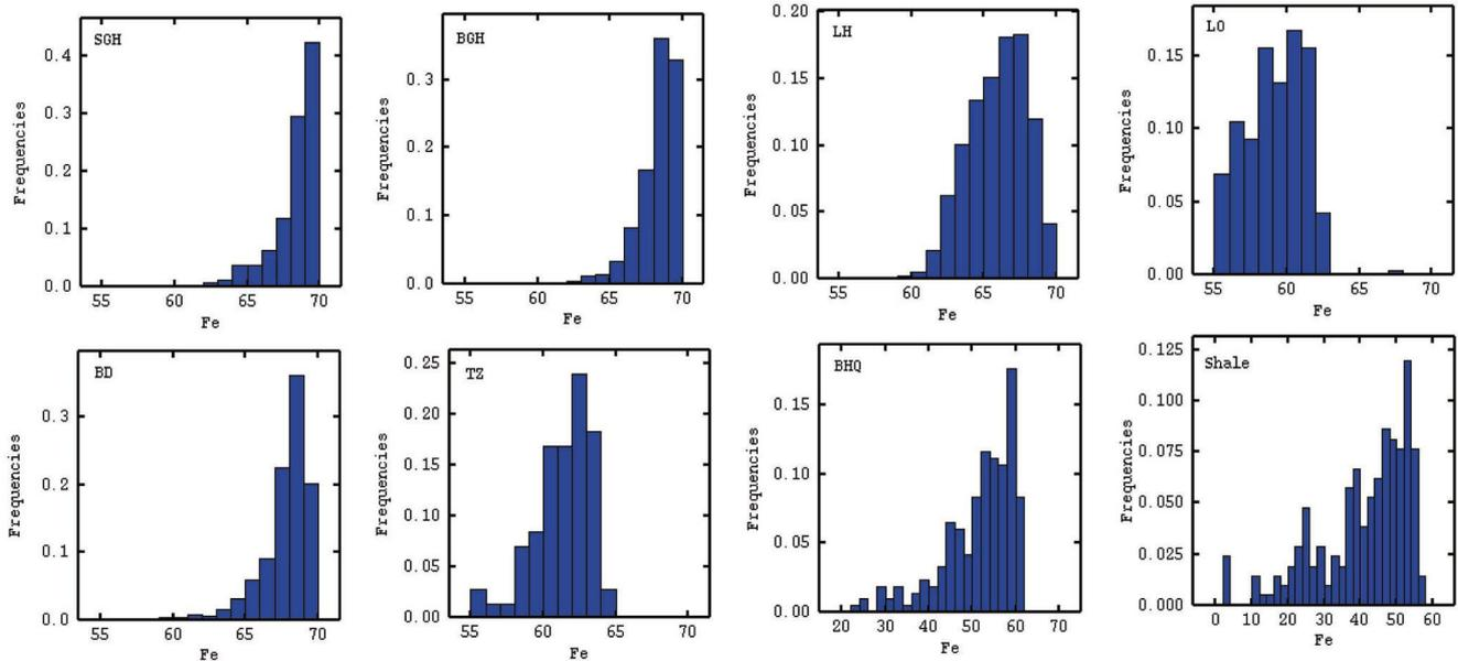
**Figure 3.** Histograms showing grade distribution of Fe% in the borehole samples of different litho units. Steel grey hematite (SGH), blue grey hematite (BGH), laminated hematite (LH), lateritic/limonitic ore (LO) and blue dust (BD) show very high-grade Fe% varying between 55% and 70%, whereas banded hematite quartzite (BHQ) and shale show low-grade Fe values.
