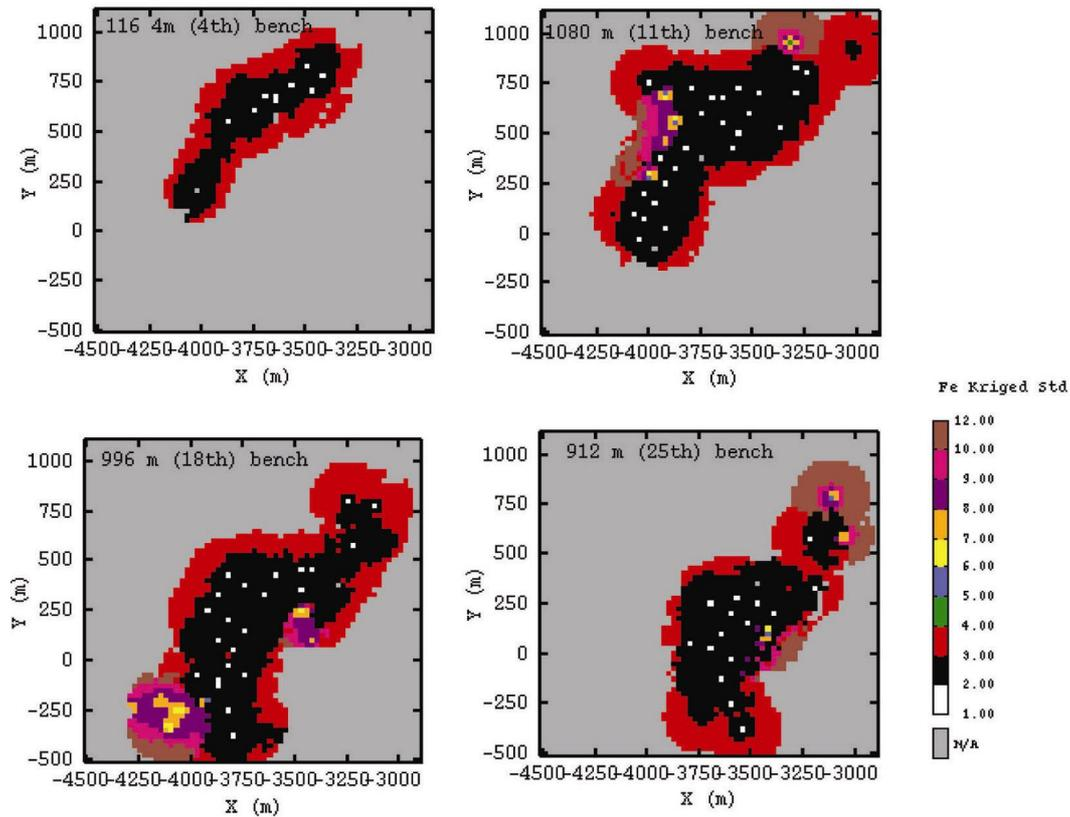
**Figure 9.** Kriged standard deviation maps for the benches located at 1164, 1080, 996 and 912 m. The central part of each mining bench has a very low grade varying between 1 and 3%. High variation in estimated grade is observed only in peripheral areas.
