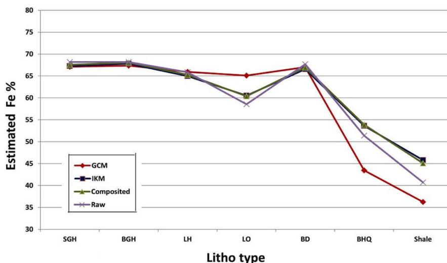
**Figure 10.** Comparative Fe kriged grade results obtained from both the methods – geological cross-sectional model (GCM) and indicator kriging model (IKM). The estimated grades match perfectly in all the litho units of SGH, BGH, LH and BD, except in LO where conventional estimation model differs from the remaining methods.
