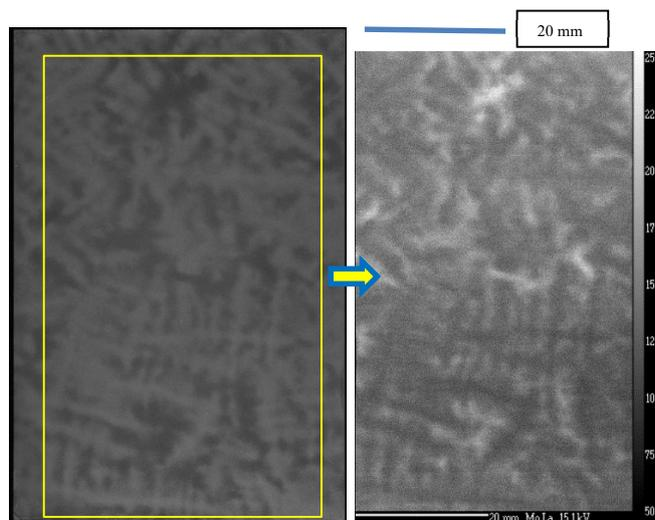
Figure 2: Comparison of a Macrograph (Nital Etching) in the S plane (Left) with a Castaing Micro-probe-mapping (Molybdenum) of the same sample (Right)
