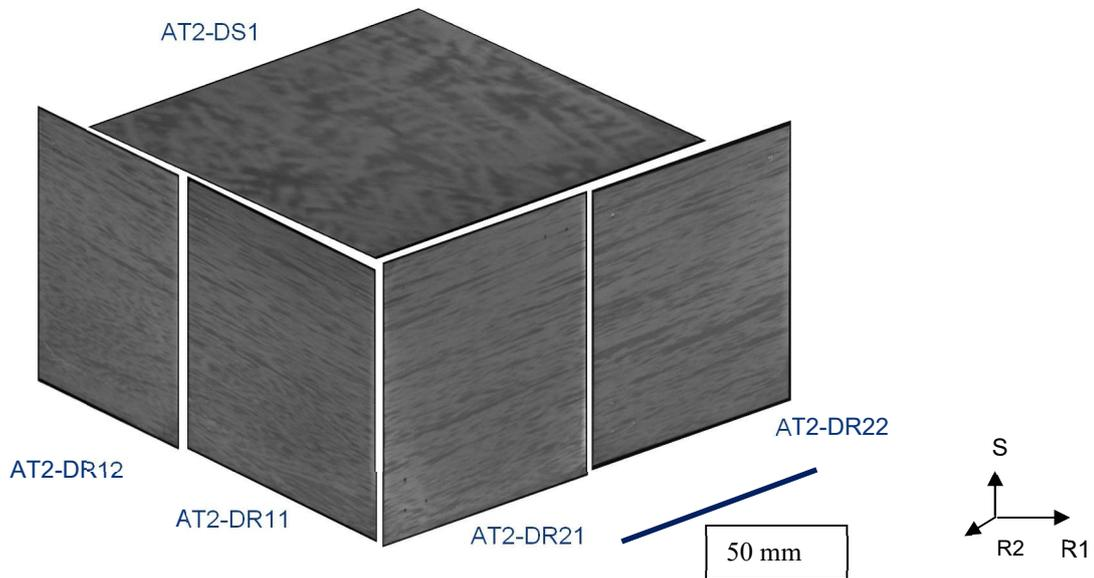
Figure 1: Macrographs of the material in 3 planes normal to the principal axes of the forging process (Nital Etching)
