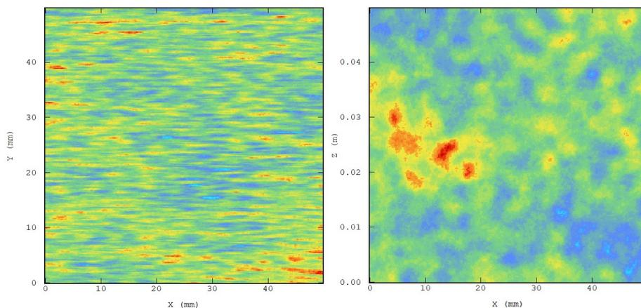
**Figure 4: Example of simulated structure of local segregation. Colour represents a normalized scale of grey level (similar to macrographs). Left section through a plane normal to R1 or R2 – Right Section to a plane normal to S**
