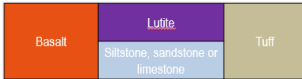
Fig. 2: Example of a lithotype assemblage rule for plurigaussian simulations
